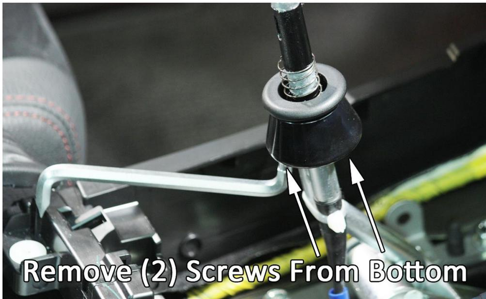
7. Apply included grease to upper and lower black plastic bushings on shift lever. Apply a small amount to inside of PERRIN Reverse Lockout Lever.
