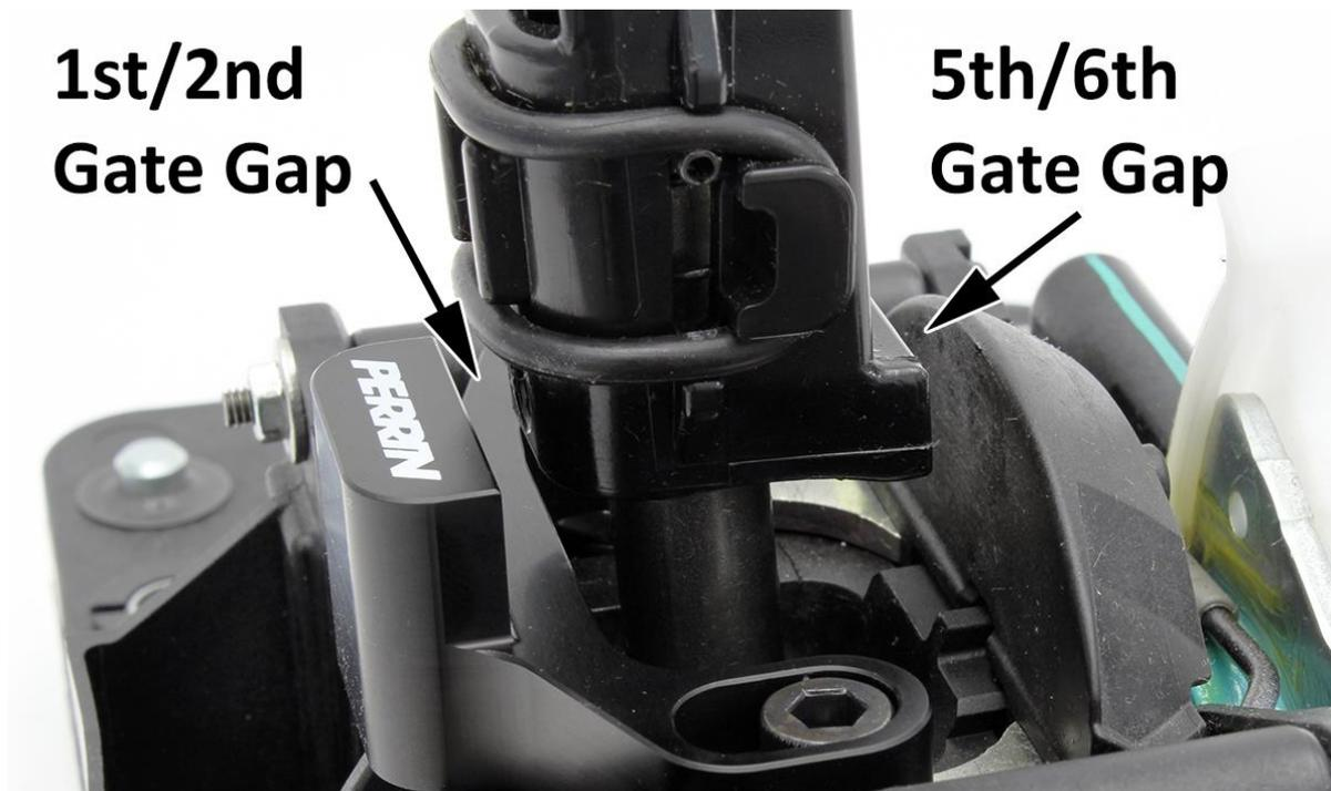
**Above picture shows shifter in neutral. Actual gaps when 1<sup>st</sup>/2<sup>nd</sup> gear or 5<sup>th</sup>/6<sup>th</sup> gear are selected, will be much smaller.**
