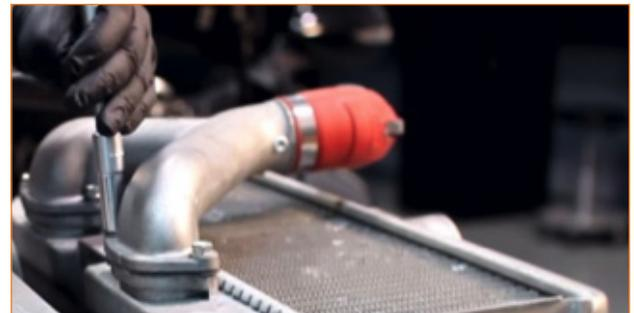
2. Reattach the stock Y-pipe to the Mishimoto top-mount intercooler using the provided Y-pipe gaskets.
