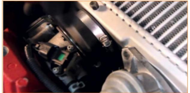
8. Remove the two driver-side bracket bolts on the intake manifold.
