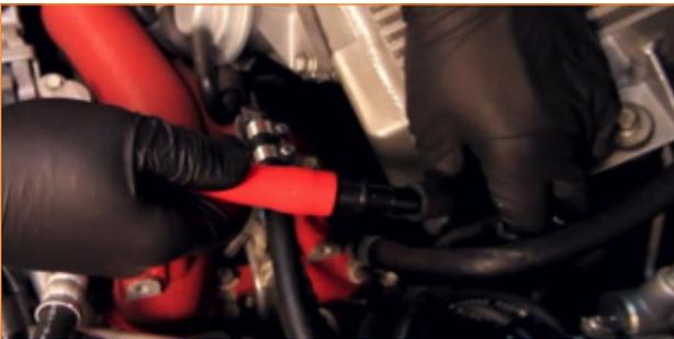
16. Connect the final two passenger-side hoses to the PCV hose.
