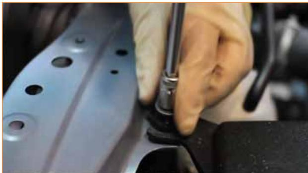
3. Once all the connections have been detached, remove the factory airbox from the vehicle.
