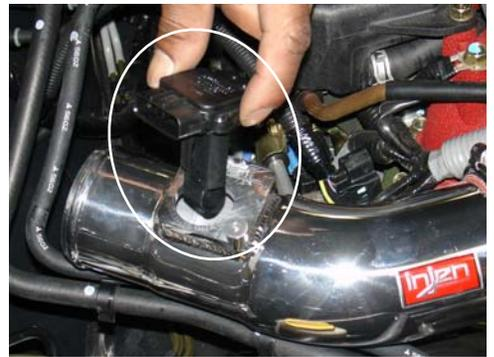
Insert the MAF sensor into the machined sensor adapter and use the same stock screws to secure the sensor in place.
