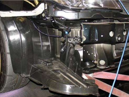
The front bumper and air intake resonator has been removed for installation of the cold air intake.
