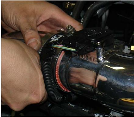
Insert intake end into the inlet side as shown above. Adjust the intake bracket to the vibra-mounts stud and semi-tighten clamp.
