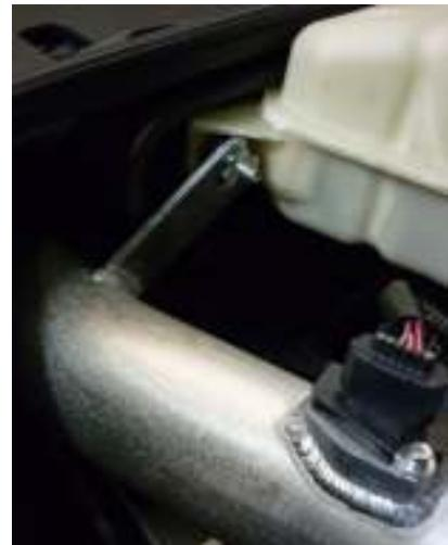
5. For the right hand side intake, remove the lower bolt on the power steering reservoir using a 10mm socket. Position the intake tube so it fits securely in the turbo coupler. Use the supplied M6 x 40 bolt, lock washer and fender washer to secure the intake tube bracket to the power steering reservoir mounting point. The order will be reservoir, bracket on the intake tube, fender washer, lock washer and finally the bolt head.
