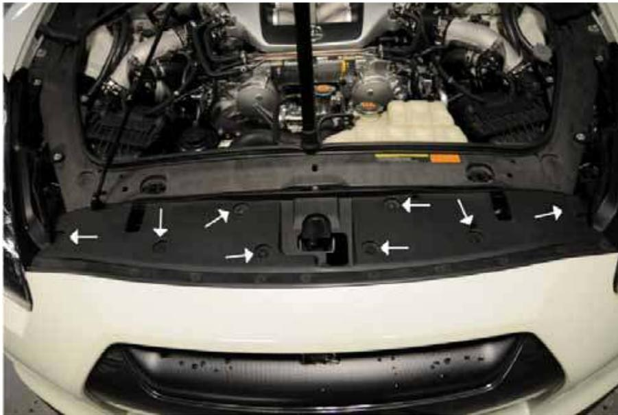
2. Starting on the left hand side of the car, use a flat head screwdriver to remove the push clip from the velocity stack along with the push clip and bolt (10mm socket) from the bracket located next to the velocity stack. Remove the velocity stack and bracket. These parts will not be reused.
