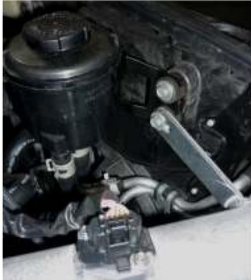
6. Tighten the clamps on the turbo inlets and intake tubes using an 8mm socket.
