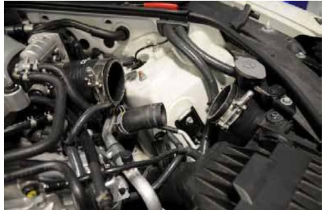
4. Disconnect the ground connection from the front timing chain case (12mm socket) and unclip the MAF sensor.
