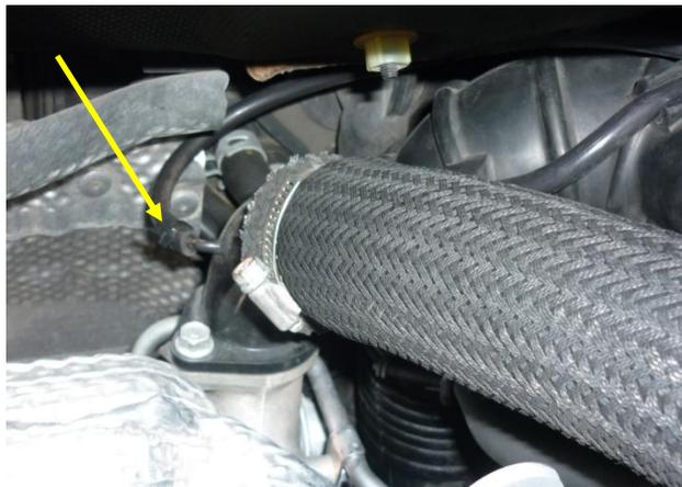
14. Ensure all lines are neatly routed and tucked with no kinks in the line all while being fully seated onto the barbs of all the connections and secure them with the included 4" zip ties. Trim the ends of the ties with scissors.
