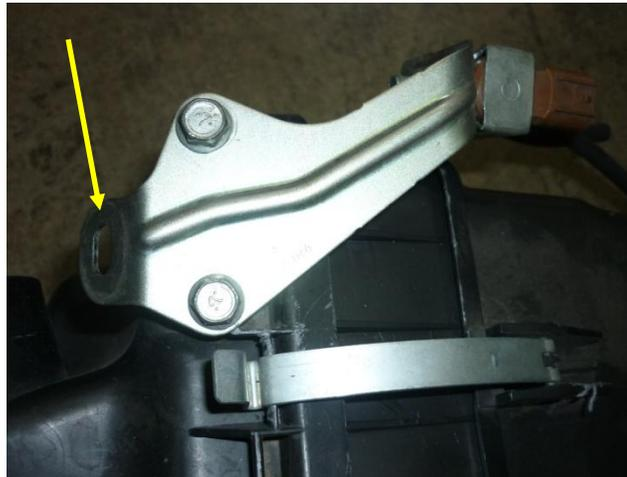
5. Using a 10mm socket, remove the two bolts that hold the bracket for mounting the factory solenoid to the airbox.
