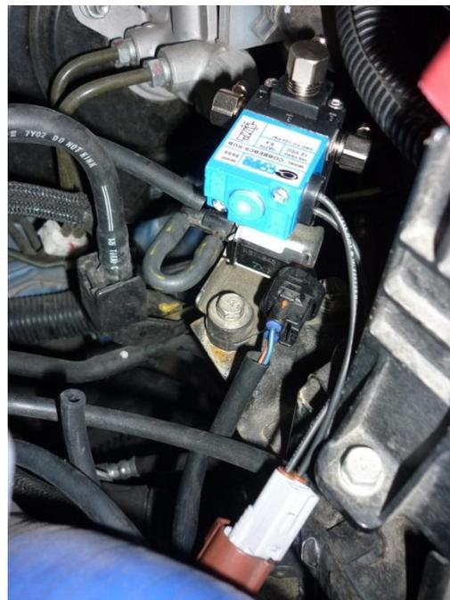
8. Remove factory vacuum lines that were previously installed onto the factory boost control solenoid from the vehicle and replace them as outlined in the following steps.
