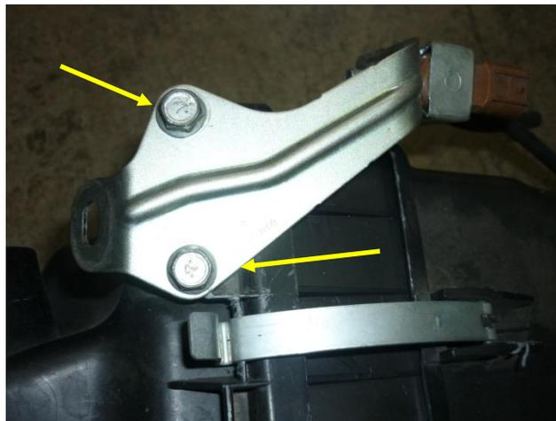
6. Remove the solenoid from the bracket using a 10mm socket.
