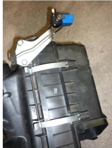
8. Reattach the bracket with solenoid to the factory airbox using the two bolts you removed and a 10mm socket.
