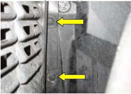
7. With the undertray removed, you will need to remove the two remaining 12mm bolts that secure the lower intercooler pipe bracket to the chassis.
