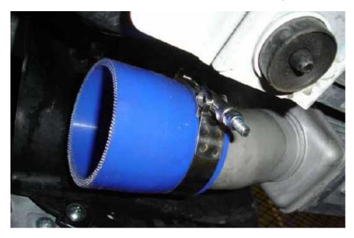
3. Slide a 2793 T-bolt clamp over the top end of the COBB hard pipe and loosely install the 45 degree 65mm to 70mm silicone reducer. Loosely install the 2794 T-bolt over the 45 degree silicone. Slide another 2793 T-bolt clamp over the lower side and install the lower intercooler pipe.
