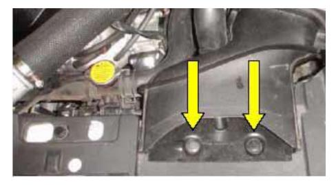
2. To remove the air box, disconnect the MAF connector and the two plastic clips that secure the MAF sensor harness to the air box. Now remove the 10mm bolt on the front of the air box. Finally, loosen the 10mm hose clamp that secures the turbo inlet to the MAF housing and lift the air box up and out of the car.
