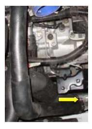
4. To make the removal and installation of the intercooler pipe easier, remove the air box support bracket. Start by removing the three 12mm bolts that secure the bracket to the chassis. Now remove the 12mm bolt that secures the factory lower intercooler pipe and unclip the wire harness from the bracket.
