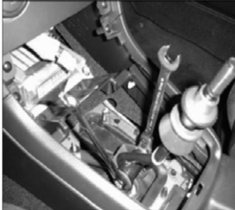
8. Cut the zip tie holding the reverse lockout cable to the shift lever.
