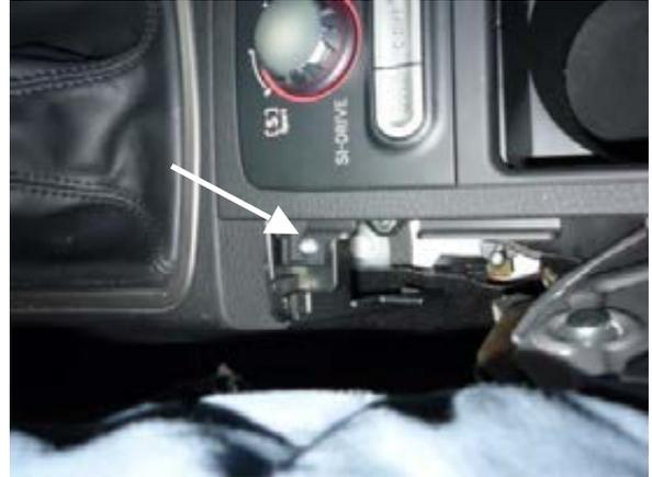
6. (08+ STi Only) Lift up on the rear of the shifter surround and slide it back towards the rear of the car. Unclip the wire underneath this piece in order to be able to set the trim piece aside.
