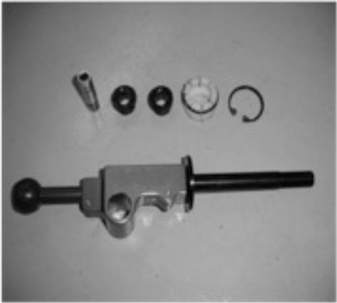
Bushing components to be re-installed
