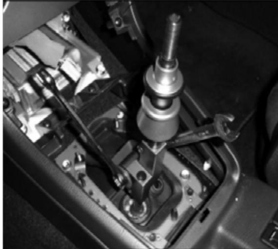
7. Thread the reverse lockout cable into the shifter's center section and into the top section. It may be easier to do this while the upper portion of the shifter is in its lowest position. You should be able to see the hole in the top of the reverse lockout cable thru the notch in the upper portion of the lever.
