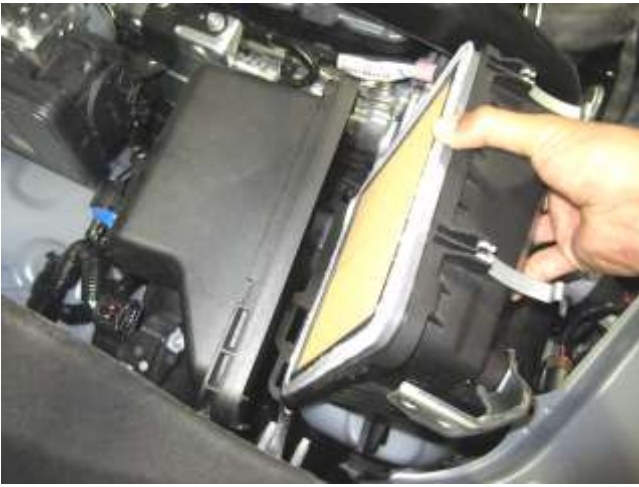
e. Unlatch and carefully remove the stock air box lid and filter from the engine bay.
