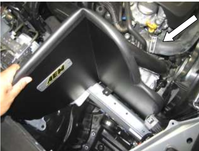
c. Install heat shield(20-8537) as shown, careful to avoid snagging high beam headlight harness.
