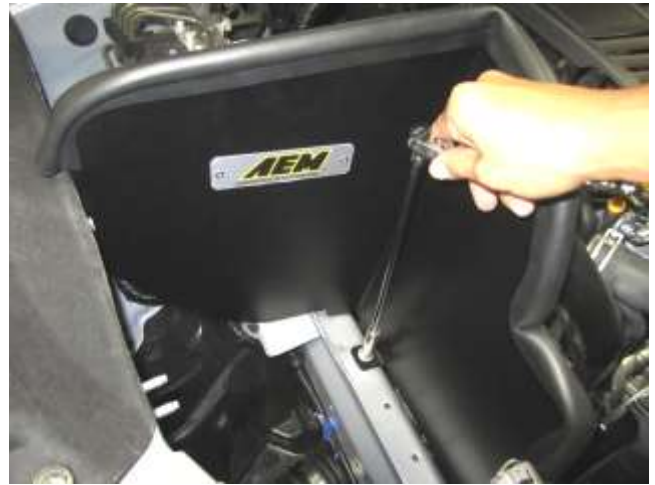
f. Use previously removed M6 bolt from 2d) to secure lower mounting tab on heat shield to frame as shown.
