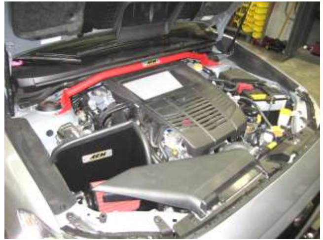
n. AEM intake installed.
