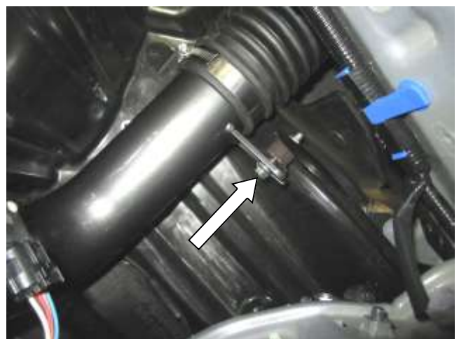
j. Use the stock nut from removal step 2f) to secure the lower intake bracket.
