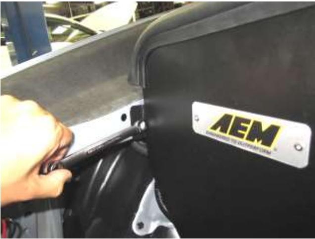
e. Use M6 bolt(22224) and crush washer(1-3025) to secure mounting tab to frame.
