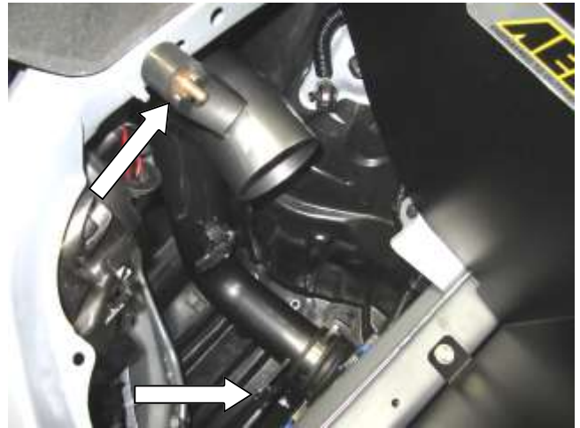
h. Insert AEM tube into lower bellow coupler and align mounting brackets as shown.
