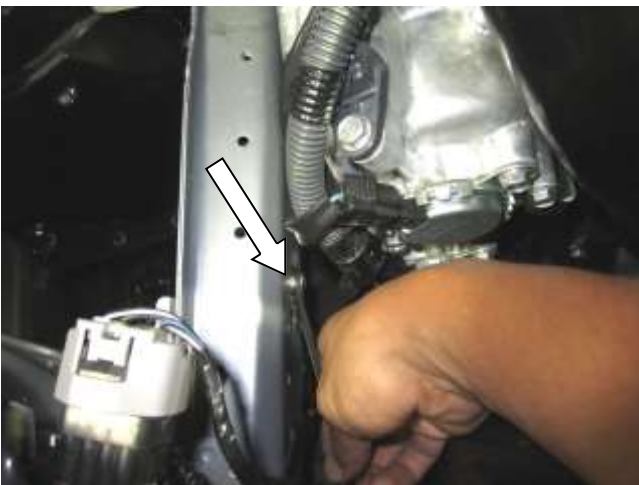
i. Remove the M6 ground bolt located on the lower frame rail and set aside for use with AEM heat shield.
