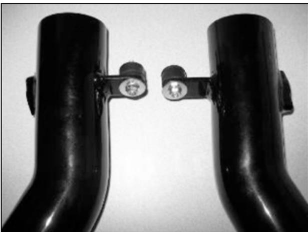
d. Install the rubber mounts on to the brackets on both pipes. Secure with a 6MM fender washer and M6 nut.
