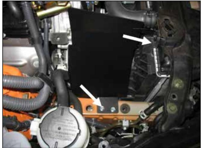
c. **Passenger side:** Insert the heat shield as shown. Secure with new hardware for the base of the heat shield and the factory radiator support bracket.
