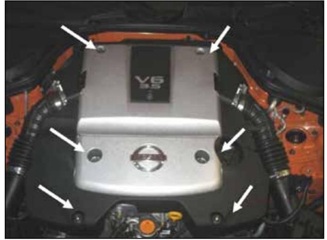
b. Loosen and remove the mounting bolts and nuts from the engine covers. Remove the engine covers.
