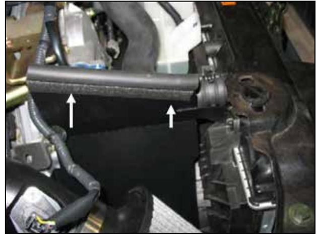
n. Insert the factory MAF wire harness clips into the oval shaped holes on the shields, this applies to both sides.
