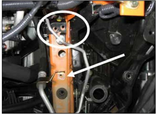
f. Loosen and remove the four A/C line bracket mounting bolts and the rubber grommet that is in between the brackets.
