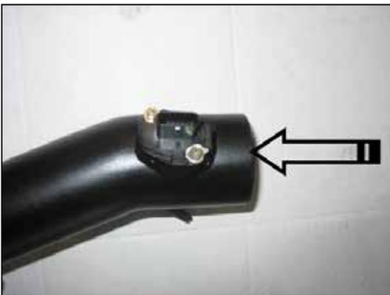
f. Remove the MAF sensors from the factory inlet tubes. Install the MAF sensors into the AEM inlet pipes, use factory hardware.
