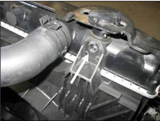
g. Loosen and remove screw that secures the radiator fan to the radiator. This applies to both the driver and passenger side.
