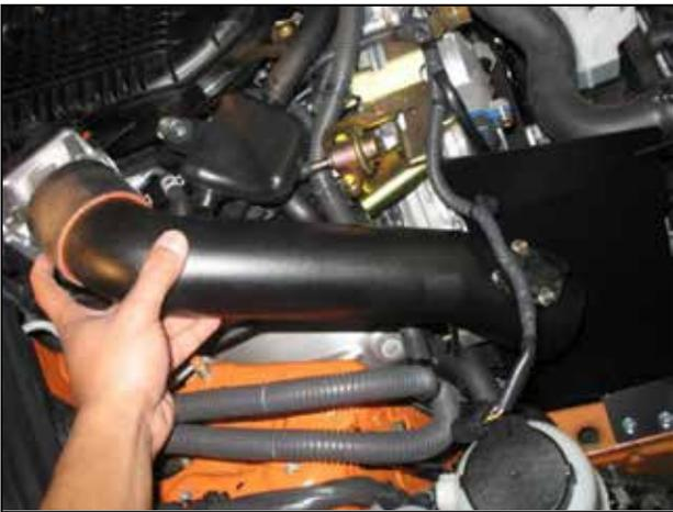
i. Push the coupler onto the throttle body.
