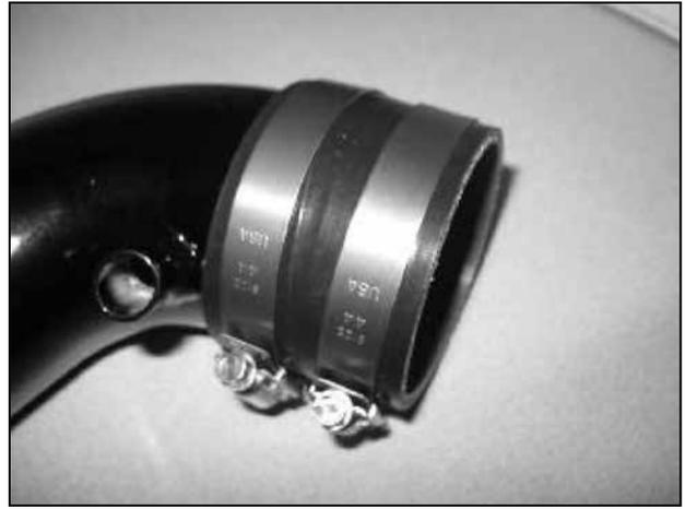
h. Insert the pipe as shown. Align the pipe bracket with the rubber mount. Then align the coupler with the throttle body.
