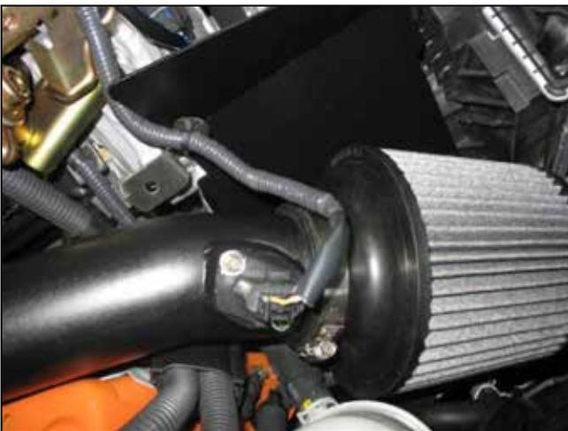
k. Connect the 5/8" hose from the crankcase vents to the intake pipes on both sides (Driver side: 1.75" length, Passenger side: 2" length). Secure with the factory clamp on the plastic nipple and a 1" hose clamp on the pipe side.
