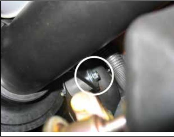
m. Attach the foam gasket to the top of the shields on both the passenger and driver side.
