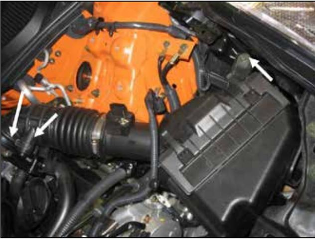
e. Loosen and remove the air box mounting bolt. Loosen the hose clamp at the throttle body. Disconnect the breather hose. Remove inlet tube and air horn mounted in the radiator support.
