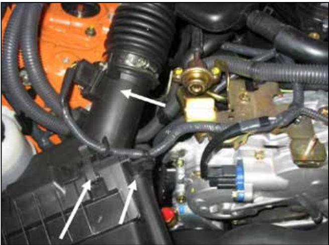
c. Unplug the Mass Air Flow (MAF) Sensor connector and unclip from the air box. Repeat for the driver side.
