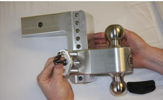
**STEP 3:** Insert the Keylock Assembly (WS03) into the 180 Slider when you have achieved the desired position along the Drawbar and lock in place by turning the key.
