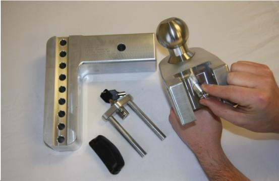
**STEP 1:** Ensure that the Ball Retaining Pin is inserted fully into the 180 slider. Do not operate without ball pin in place.
