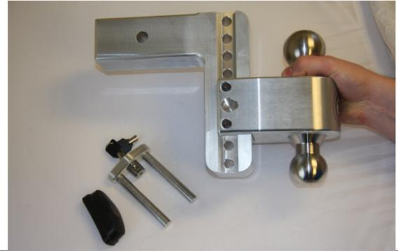
**STEP 2:** Place the 180 slider at the desired drop on the Drawbar in order to ensure that your vehicle and trailer are properly positioned.
