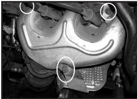
Step 13. Install the passenger side heat shield using the remaining two flange bolts and heat shield brace bolt.
