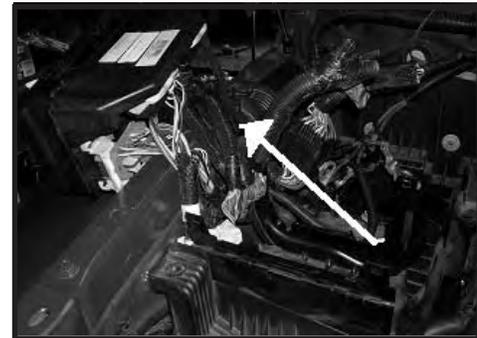
Step 8. Once the fuse box tabs have been released, lift the box up and lay it over the side of the fender. Remove the large plastic tray and set aside. Remove the spark plugs wires from the plugs only and label each wire.
