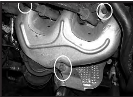
Step 9. Remove the passenger and driver side heat shield bolts. Remove both heat shields. Do not discard the passenger side, it will be reused later. A bolt penetrating spray may be needed.
