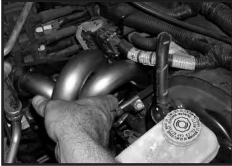
Step 11. Install the driver side header, and gasket. The header will have to be angled down when installing. Install the upper flange bolts with a small amount of thread locker applied. Use caution installing the manifold bolts into the aluminum head. Torque bolts to 20 ft-lbs.
