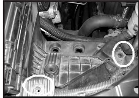
Step 6. Remove the two front tray mounting bolts.
