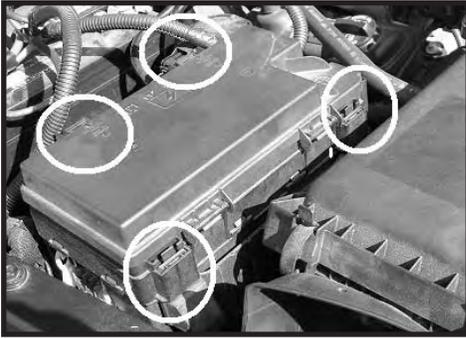
Step 7. Remove the fuse box by pressing the four release tabs located on each corner of the fuse box.
