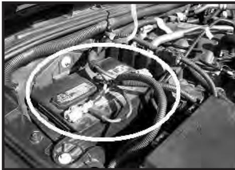
Step 1. Disconnect the battery terminals from the battery and move aside. Remove the battery hold down clamp. Remove the battery.
