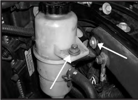
Step 5. Remove the power steering reservoir bolt and move the reservoir to the side. Remove the reservoir mounting bracket and set aside.
