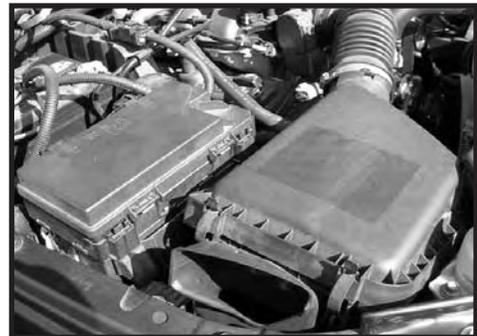
Step 16. Reinstall the battery tray, battery, power fuse box, steering reservoir and bracket, and air box. Start motor and check for exhaust leaks.
