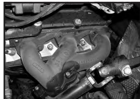
Step 10. Remove the two down pipe flange bolts on each manifold. Remove the remaining bolts holding on each manifold. Remove both manifolds and set aside. Remove any remains of the old gasket material that is left on the head. Be careful not to gouge the aluminum cylinder head.
