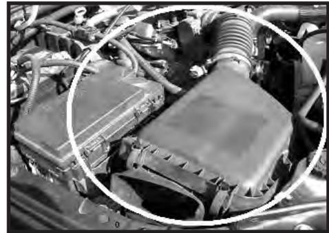
Step 2. Remove the PCV hose from the filter box. Remove the air filter cover by unclamping the cover and removing the hose clamp on the throttle body. Remove the air filter, and housing. The housing is held in by three rubber grommets on the bottom of the box. A rocking motion may be needed for removal of the air box.
