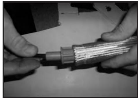
Step 14. Install the heat shield boots on all of the plug wires. The longer boot goes on the #6 driver side rear plug wire. Reinstall all the spark plug wires on the spark plugs.
