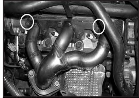
Step 12. Install the passenger side header, and gasket. Install the upper flange bolts with the exception of the top left and right bolts. These bolts will be used to hold the factory heat shield in place. Install the down pipe flange bolts on each side
